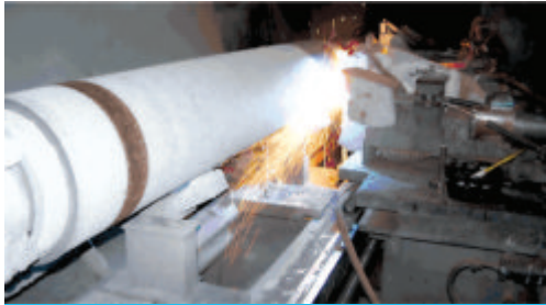
PRO-COMARC® coating system consisting of 2 wire feeder, sprayer, DC Plasma Arc device
