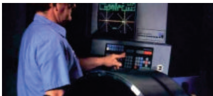
To assure reliable, vibration-free performance, all Xtek brake wheels are dynamically balanced on sophisticated, computer controlled testing equipment.
