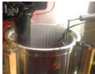
Coupling ring gear during finish grinding of the internal gear teeth.
