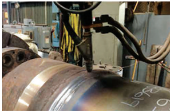
Coupling adapter and spindle weldment assembly, during the submerged arc welding (SAW) process. In many cases reconditioned gear coupling assemblies requires that replacement components are joined to modified components. All welding processes at Xtek are tightly controlled and utilize superior welding wires and flux combinations to produce the desired metallurgical properties.
