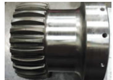
Splined coupling adapter and hub gear at final inspection
