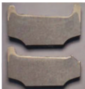
Cross sections of a competitor's wheel graphically illustrates the perils of brittle, through hardened flanges.
