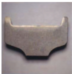
Xtek track wheel cross section demonstrates its hardened contour case (S88-62 Rc), backed by a ductile support zone in both flange and tread.
