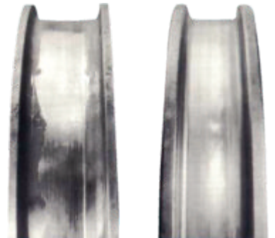
After 3,000,000 cycles, a competitor's wheel shows severe spalling, irregular wear and a deep groove. On right, The Xtek wheel shows no visible signs of wear after more than 12,000,000 cycles.
