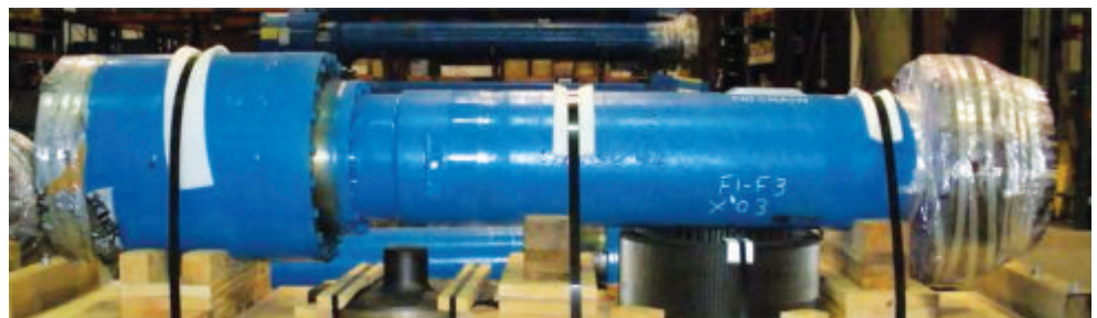
HSM F1-F3 Gear Coupling X-03, along with DE Thrust Plate and DE Ring Gear, ready for shipment.
