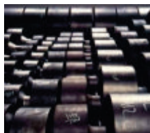
Xtek forged steel brake wheels after heat treating and inspection, ready for final machining.
